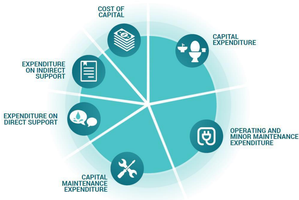
Figure 1 The six life-cycle cost categories for sustainable WASH service delivery
